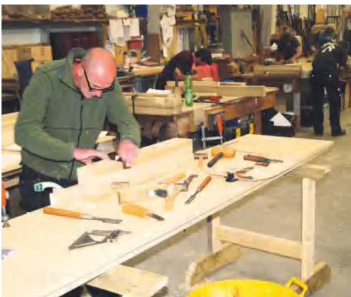
▲ Pic.11 Another view of cleaning up the laps. Note the small number of tools on the bench. It is not how many tools you have but how you use them that counts
